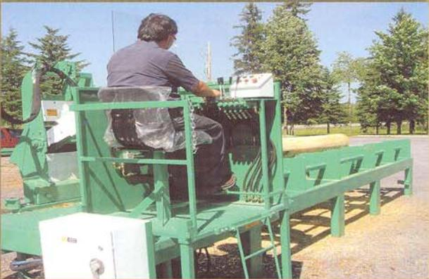
Foot controlled carriage movement allows hands to be free for hydraulic controls.
