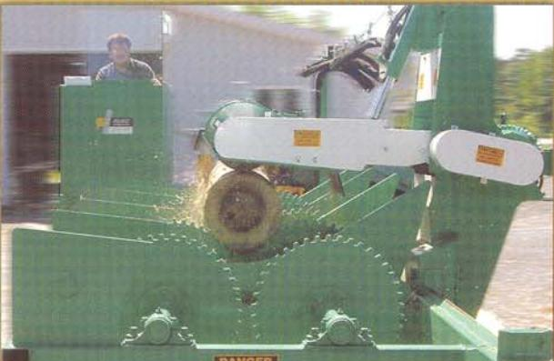
Model 36 is equipped with a 12" debarking head with carbide teeth and built in depth control. The 20 hp electric motor allows for vigorous performance while it runs at an optimum 1700 RPM for both speed and cost efficiency.
