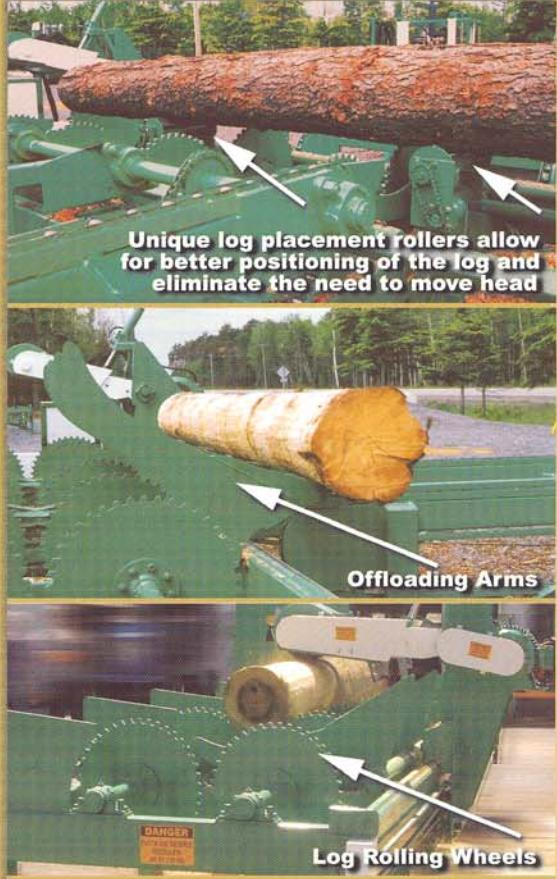
The hydraulic system features a 16 GPM tandem pump powered by a 15 hp electric motor. Log handling capabilities are extensive with 12 log rolling wheels, 4 unloading arms, 2 log placement rollers to forward or reverse log and 2 hydraulic plugs for (optional) infeed deck.
